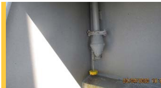
SHOWING A COAMING DRAIN VALVE WITH THE FIRE CAP PROPERLY CONNECTED TO THE VALVE WITH A LANYARD.
