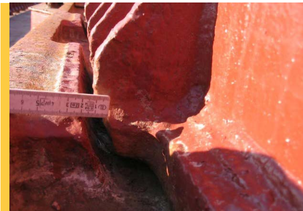
MEASURING EXCESSIVE CLEARANCE IN WAY OF A TRANSVERSAL (FY) STOPPER.
